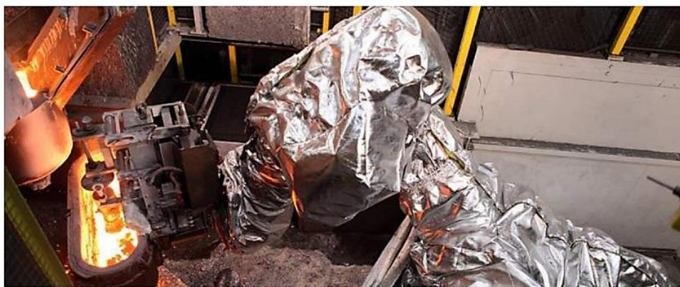
Рис. 11. Robotic aluminum cover jacket that suits foundry and forging
