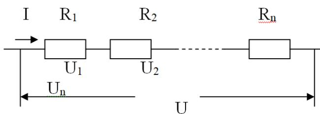
$$\begin{aligned} I &= \text{const} \\ U &= \sum U_i \\ R &= \sum R_i \end{aligned} \quad (124)$$
